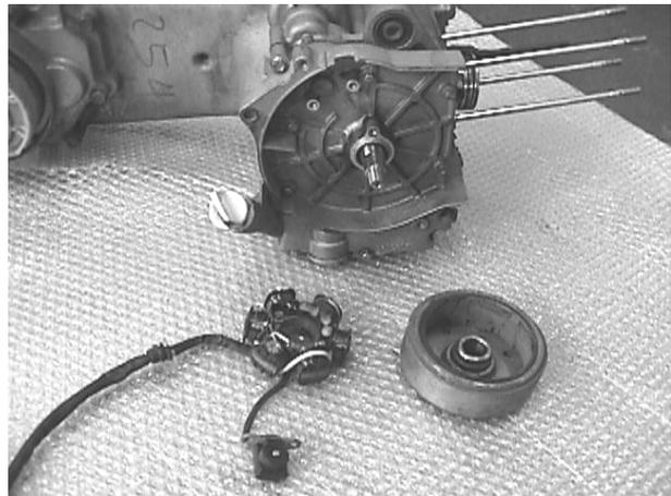
6. Remove the washer, lock pin
