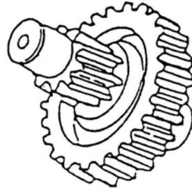
3. Check the wearing condition of the final reduction gear.
