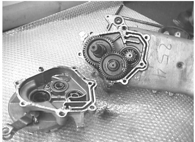
4.Remove the final reduction gear
