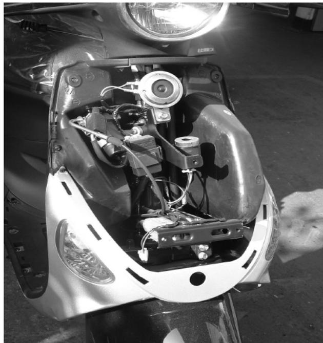
D.Dismantling the step plates and lower
