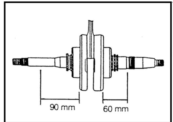
3. Check the looseness of crankshaft bearing.
