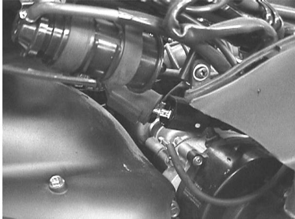
3. Check regulator measure the resistance value between each terminal, it should be in specified range, otherwise change a new one.
