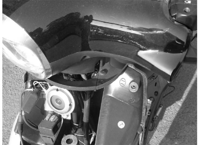
E.Dismantling the step floor and front
