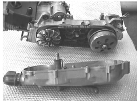
2. Remove the lock nuts of driving Plate and the nuts of Starter gear And clutch.
