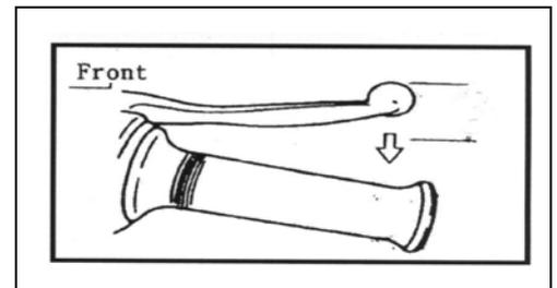
Note: Try brake lever to see if it's loose. Check the brake oil. Once air mixed in the oil pipe, which will reduce or damage the brake efficiency or even its function.
