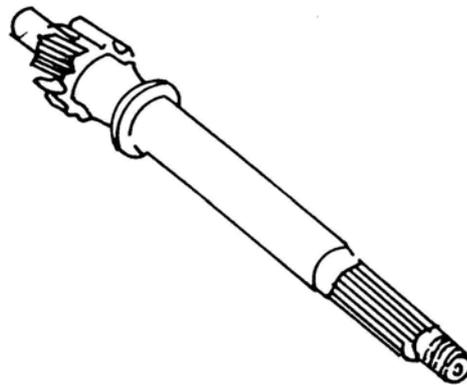
2. Check the wearing condition of idle gear shaft and idle gears.
