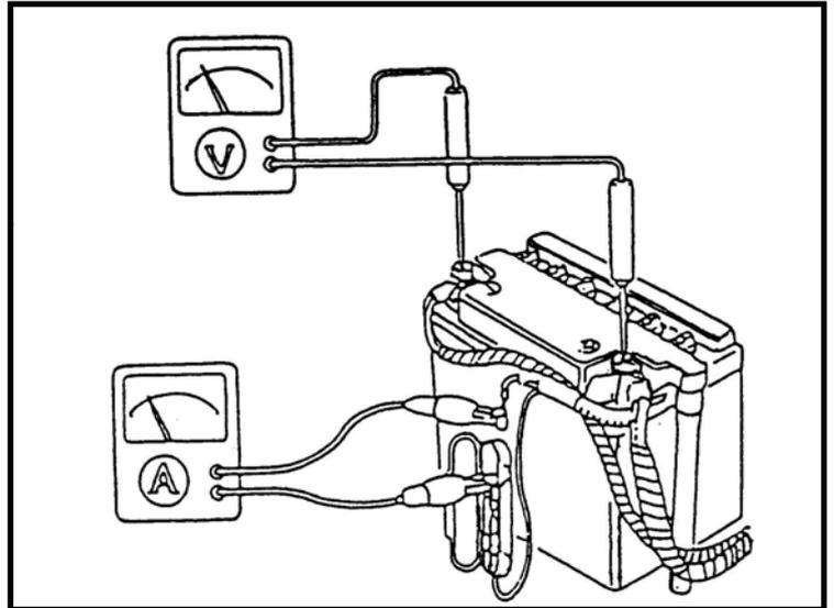
While testing, the red wire cable must not touch the frame.
