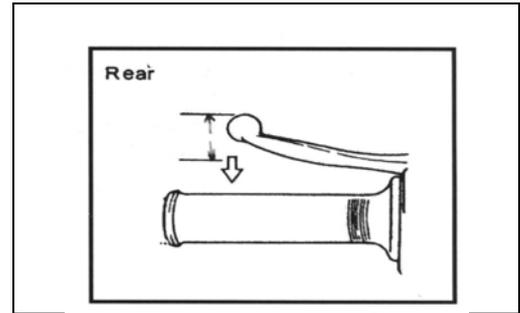
Note: When the arrow of rear brake indicator align with the arrow of left crankcase, change the brake lining.
